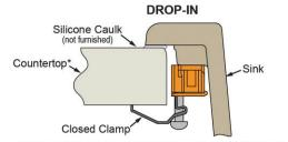
\*Maximum thickness for use of hold down system is 1-3/4" (44mm).
