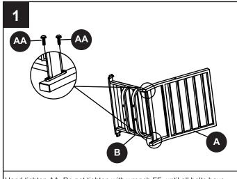
Hand tighten AA. Do not tighten with wrench FF, until all bolts have been installed.
