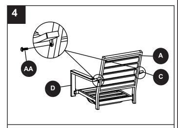
Hand tighten AA. Do not tighten with wrench FF, until all bolts have been installed.
