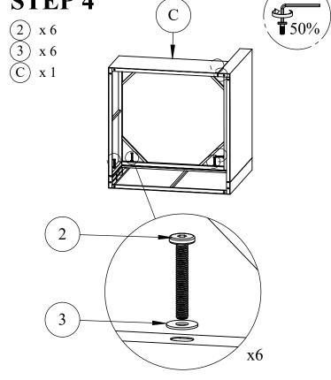
Connect part from STEP 3 & Seat Corner (C) with Bolt (2) & Washer (3).
