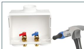
Figure A-2. Knockout Instructions: Do not attempt to knockout test caps before securing outlet box to drain pipe.
