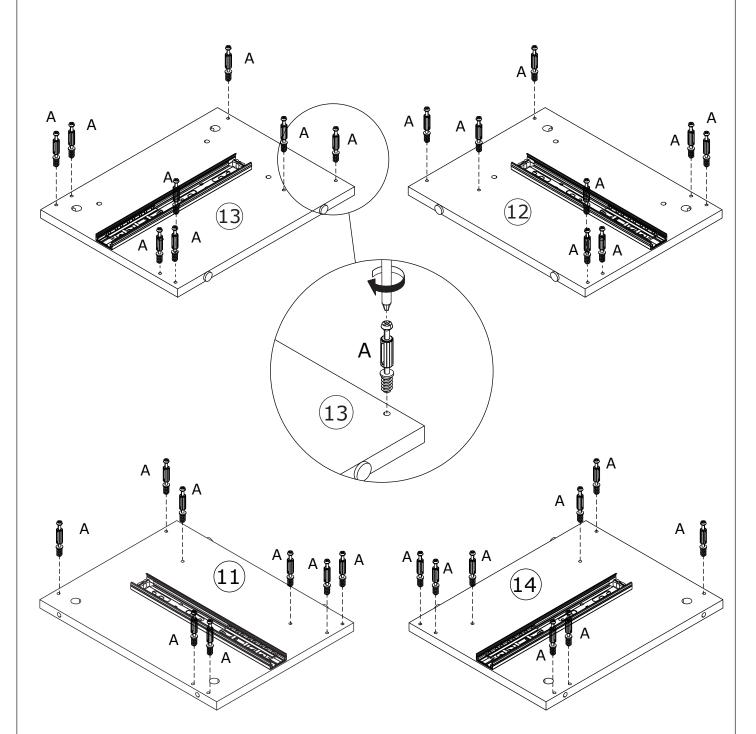
Screw eccentric rod(A) into board 11, 12, 13 and 14 at first.
