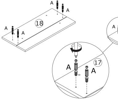
Attach board 17/18 to board 19 and 20, add cam lock(B) into and turn clockwise to tighten as shown.
