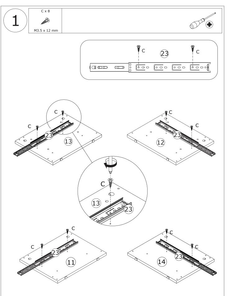
Fix rail 23 to board 11, 12, 13 and 14 with screw(C) at first.
