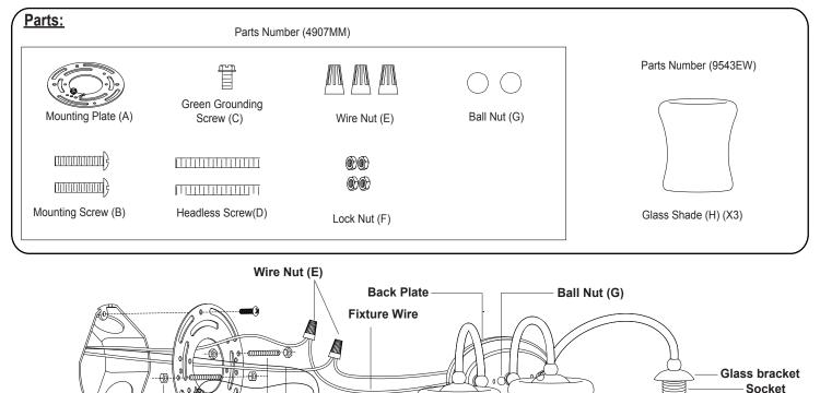
Thread two headless screws through the mounting plate, then secure them with four lock nuts (two on each side of the mounting plate). Adjust the length of the headless screws if necessary. Note: Make sure that the headless screws are lined up horizontally, to ensure that the fixture will be level.
