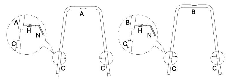
Put Upper 'U' Tube (A) into the groove of Lower 'U' Tube (B).
