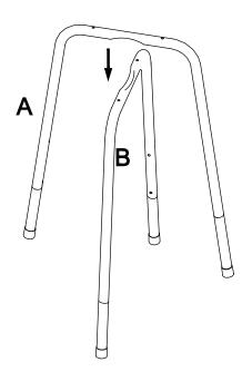
Turn the Swivel (D) 45 degrees (as picture shown) for easy assembly. Then put it on Upper/Lower 'U' tube (A) & (B), align the holes and firmly tighten with Bolt (I), Spring Washer (L) and Metal Washer (M) using Allen Wrench (N).
