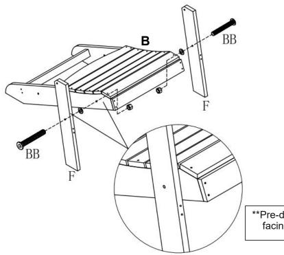
\*\*Pre-drilled hole on front leg facing front.
