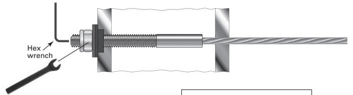
2. Tension all cables to desired amount in sequence, beginning with the center cables, moving up and down toward the top and bottom. As you tension each cable, give it a sharp pull downward mid-span to help set the wedges, then re-tension as necessary in the same sequence. Be aware that the cable may move as much as 3/16" toward the tensioning terminal as the wedges seat.
