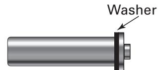
3. Rotate the Pull-Lock<sup>®</sup> fitting clockwise as you push it onto the cable. If the cable begins to "unravel," you are rotating the fitting in the wrong direction.
