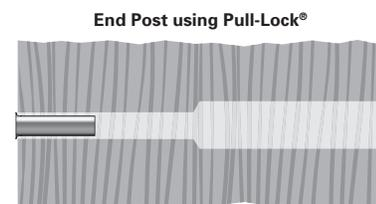
2. If using metal posts, start by inserting the plastic stud bushing into the pre-drilled hole in the post. Slide the stainless steel washer onto the threaded stud (smaller for metal post, larger for wood) and start the brass locknut onto the threads as far as possible by hand. Feed the cable through the end post, pulling the threaded stud into place.
