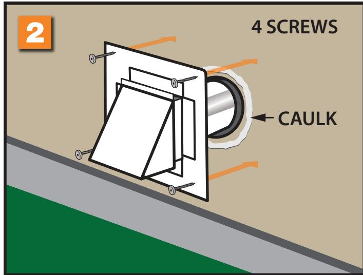
2) Apply a bead of caulking around the hole then insert the dryer vent (DV4). Affix the vent with 4 screws through the flange.
