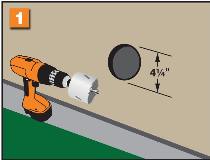
1) Drill a 3/8" hole from the inside to locate the position of the dryer vent. Note: your dryer vent should be at least 3 feet away from the nearest window or door. Cut a 4 1/4" diameter hole with a hole saw.
