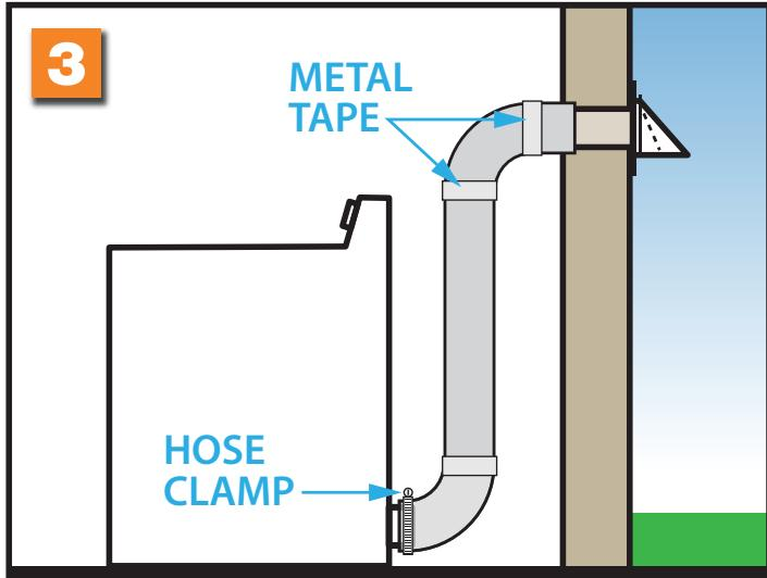
3) Assemble 4" ducting from the vent to the dryer exhaust port. Secure each component joint (ducting, elbows) with metal foil tape; do not use screws as they will trap lint. Support the ducting by securing it to joists or studs with Plumber's Tape (pipe strap).
