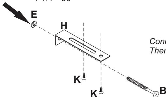
Connect the hardware (H) onto the wall with hardware (B).
