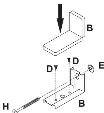
Connect the hardware (B) onto the wall with hardware (H). Then fasten with the hardware (D) the hardware (B) on the parts (02).
