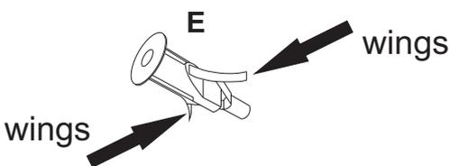
Press the hardware wings (E) to put in the hole that you drilled in the wall.
