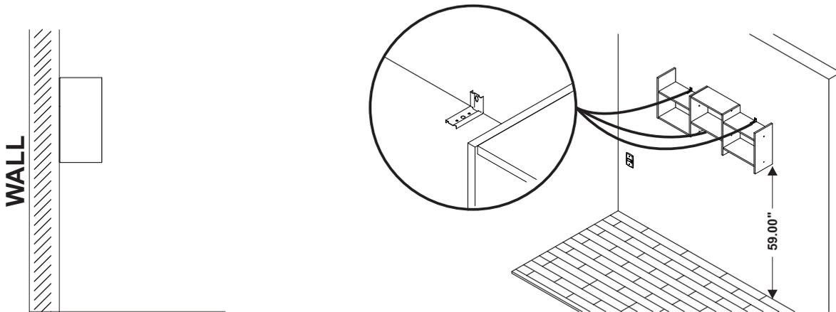
Position the hardware (B) onto the part (02) as shown in the figure. You will need a pencil to mark where you should drill the wall with a 3/8" drill bit to put in the hardware (E).
