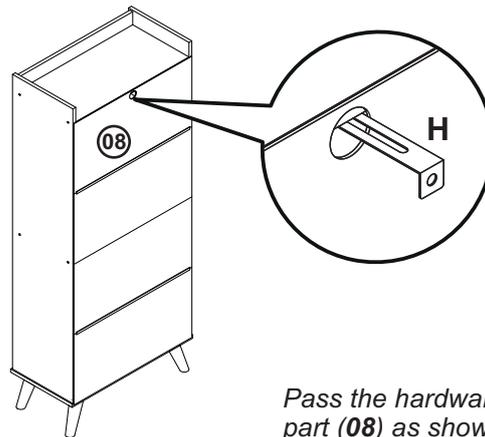
Pass the hardware (H) through the hole of the part (08) as shown in the figure.
