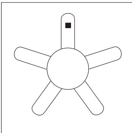
Glue the counterweight to the height of the clip on the surface of the blade. Remove the clip and test the fan. If you keep staggering, put another counterweight. If it gets worse, try another better area to place it.
