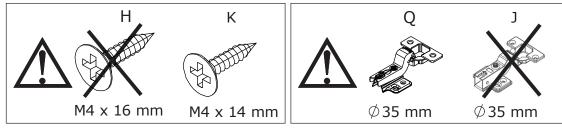
Attach board 12 to board 4 by fixing hinge(Q) with screw(K) as shown.
