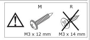
Fix back board 8 and 9 with screw(M) as shown.
