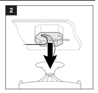
Attach mounting plate (B) to outlet box (not included) using the existing washers and outlet box screws or the machine screws (BB).
