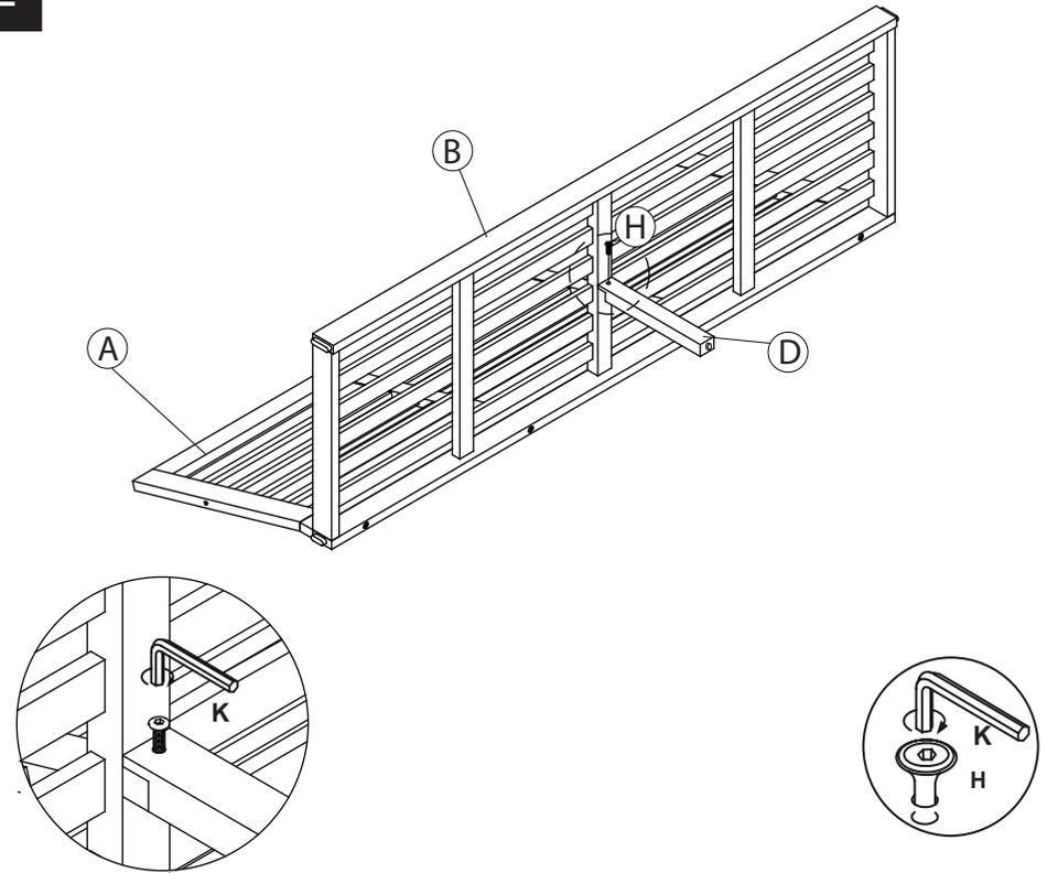
Step 2 Tighten bolt (H) with allen key (K) to attach Leg extra (D) and seat frame (B).
