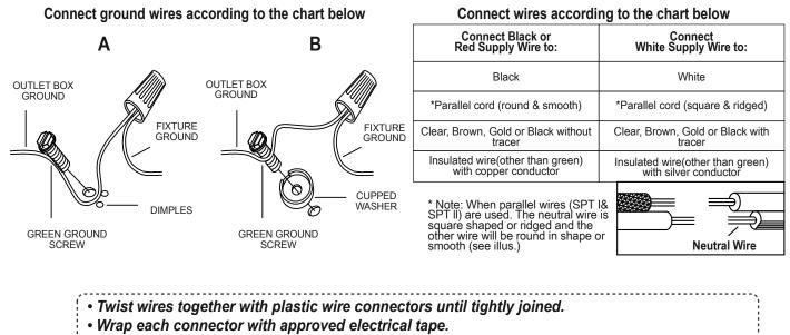
• Be sure that no wire strands are exposed and then carefully tuck all wires into the outlet box.
