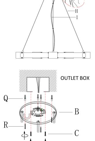
Connect wires as shown in the charts below. *PLEASE NOTE THAT GROUND WIRE IS BARE COPPER WIRE, NEVER CONNECT OTHER WIRES TO GROUND WIRES.*
