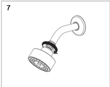
7. Install showerhead use teflon tape on at least the first 3 threads and screw on the shower head using a wrench.
