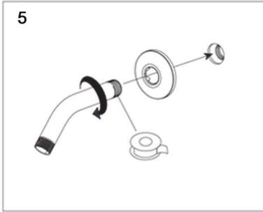
5. Install the shower arm and flange. Slide the flange onto the shower arm and teflon tape at least the first 3 threads of the end going into the wall (pipedope is recommended also for any connections in the wall) tighten arm securely.
