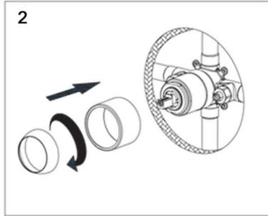
2. Install valve body sleeve and sleeve cover.
