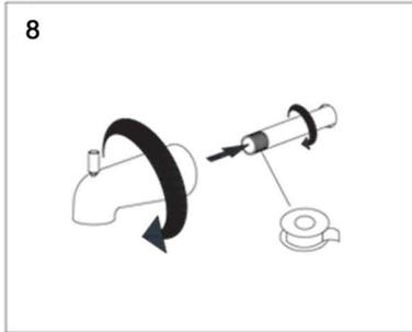
8. Install tub spout use teflon tape on at least the first 3 threads and screw on the tub spout securley.
