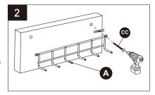
3. Re-screw toggle end to toggle bolt (CC) and insert both toggle ends into drilled holes. Tighten toggle bolts (CC) to secure to wall.
