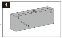
2. Drill 1/4 in. hole at screw hole marks and insert anchor (BB).
