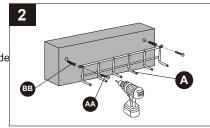
3. Using screws (AA), secure the hang-up (A) to the wall by screwing into the anchors (BB).
