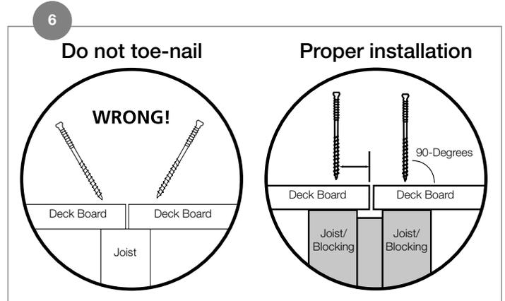
Always drive in surface fasteners at a 90° angle to the decking surface with two fasteners at every joist location. Do not toe-nail screws into the joist. Instead, place blocking/sister joists to allow perpendicular installation of surface fasteners at board ends.
