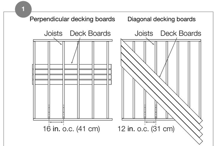
Joist location is important for the safety of the deck and will affect the layout, cost, and ease of installation for the railing system. If railing will be installed, determine rail post placement prior to joist construction. See page 9 for information about planning post placement for rail installations. Joists used in deck frame construction should be 2 in. x 8 in. (5 cm x 20 cm) or larger.
