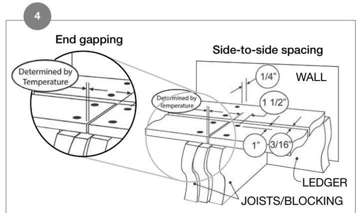
All decking materials, whether wood, composite, or metal, undergo some degree of linear expansion with the changes of weather and the seasons. For best spacing results, keep boards out of direct sun during storage and cutting processes, and throughout installation if possible. Never cut and install boards in direct sunlight. To compensate for the effects of contraction and expansion, use short boards (where possible) with splitter/divider boards between each continuous run of boards.
