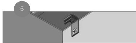
After positioning the last deck board in place, secure the deck board by angling a screw through the clip and into the board at a 30°- 45° angle. Ensure the screw inserts fully and pulls the board down (2). Space no more than 12 in. (30 cm) apart.
