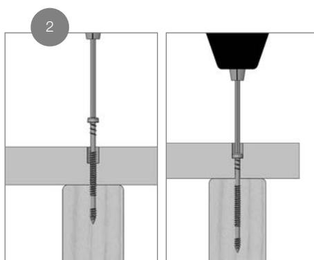
Using the Cortex setting tool, drive the fastener to the preset level below the deck surface, ensuring the fastener remains perpendicular to the deck surface. Install two fasteners at every joist and/or stair stringer. Overtightening will induce cracking at fastener locations.
