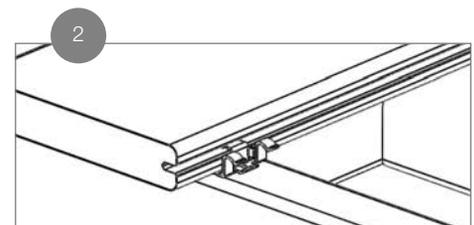
Insert a Fibron PhantomGT fastener into the groove of the board, centering on joists.
