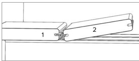
Position the next deck board into the fasteners. It may be helpful to angle the board slightly to fully seat it into the fasteners.
