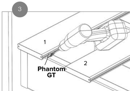
Secure fasteners by driving the screw fully into joist. Continue installing and securing the fasteners in the center of each joist along the remainder of the deck board.
