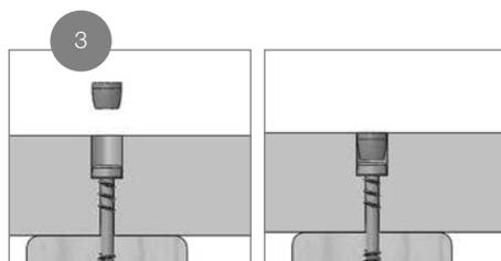
Ensure the cored hole is free of debris or moisture. Place the Cortex plug into the cored hole and gently tap with a smooth hammer head until it is flush with the deck surface.
