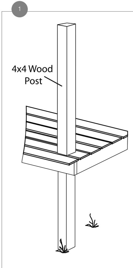
Ensure 4 in. x 4 in. (10 cm x 10 cm) wooden posts are secured in a code-compliant manner, and, where possible, spaced equally for the best looking application.
