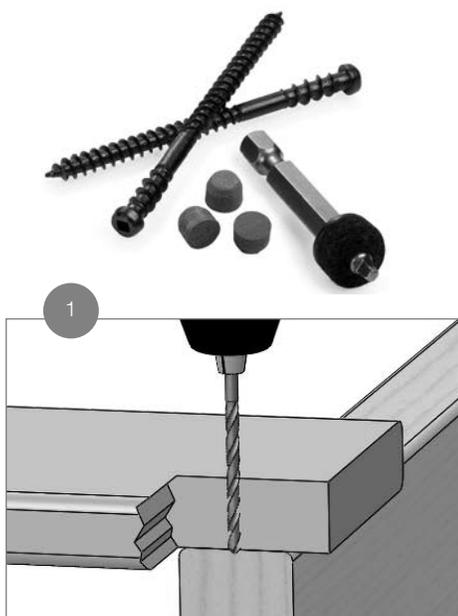
Locate all fastener holes at least 1-1/2 in. from board ends and 1 in. from board sides. To prevent cracking at fastener locations, pre-drill all holes with a 1/8 in. or 9/64 in. drill bit perpendicular to the deck surface to create the proper pilot hole and remove excess material.
