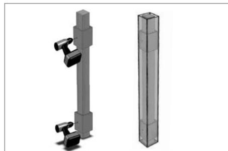
Horizon guard rail 5-3/4 in. post sleeves require adapters to be installed over the wooden 4 in. X 4 in. posts prior to installing the post sleeve.
