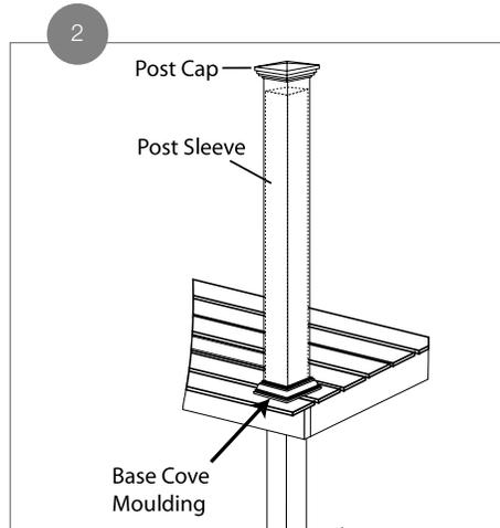
Determine the desired height of the post sleeve. Typically, the height is no less than 2 in. (5 cm) above the top of the finished guard rail system. This ensures the proper placement of the post caps that fit over the top of the post sleeve. Cut the post sleeve to the desired height.
