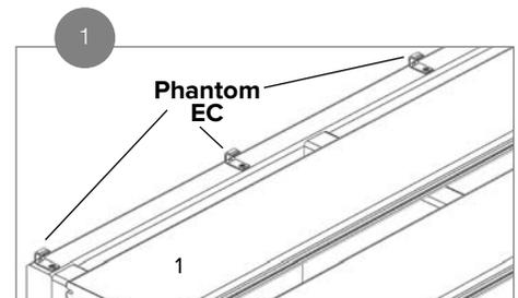
Secure Fibron PhantomEC end clips a minimum of 1/4 in. from the wall with a single screw into the joist. Space clips no greater than 12 in. apart. Position the deck board into the end clip fasteners. It may be helpful to angle the board slightly to fully seat it into the clips. Check to ensure that the board is fully inserted into the clips.
