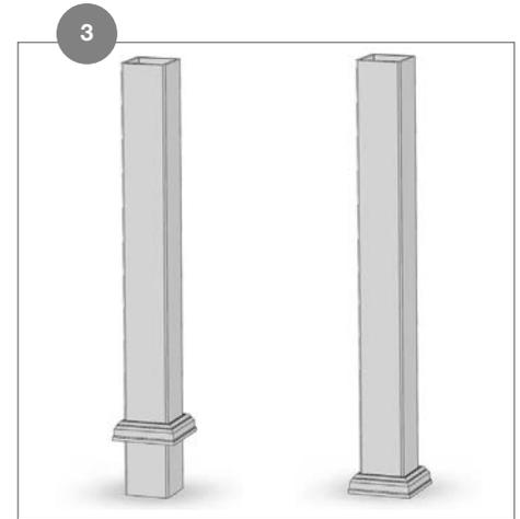
After decking is installed, slide post sleeve and moulding over the wood 4 in. x 4 in. (10 cm x 10 cm) post.
