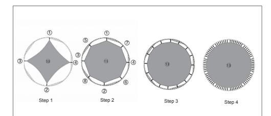
**Note:** To ensure even tension and prevent issues with subsequent spring installation, install the springs diagonally. For example, begin at the 12 o'clock position and then at the 6 o'clock position.
