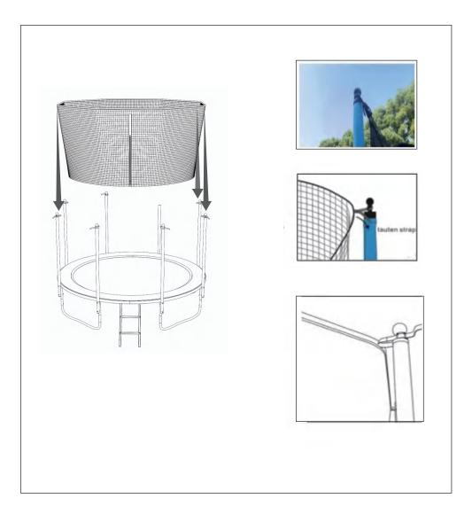
**Step 11**Components Net Ropes (#10),Safety Net(#9)through the bottom hole components,and parts cross around spring, and fixed.As shown in fig.
