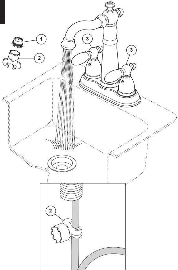
Remove aerator (1) using supplied wrench (2) and turn faucet handles (3) to the full on mixed position. Turn on hot and cold water supplies (4) and flush water lines for one minute. **Important: This flushes away any debris that could cause damage to internal parts.** Verify the seal is attached to aerator then reinstall. **Note: For future use, aerator wrench (2) can be clipped to the supply line after flushing faucet.**
