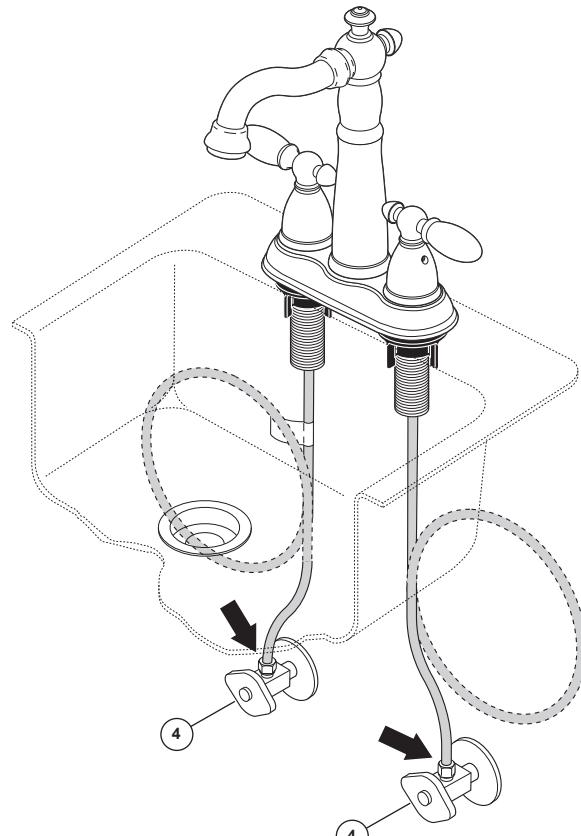
Check all connections at arrows for leaks. Re-tighten if necessary, but do not overtighten.
