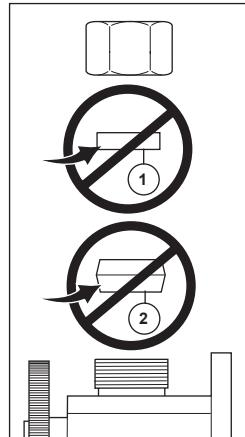
**Do not use gasket (1) supplied with PEX tubing or brass ferrule (2) supplied with valve stops.**
