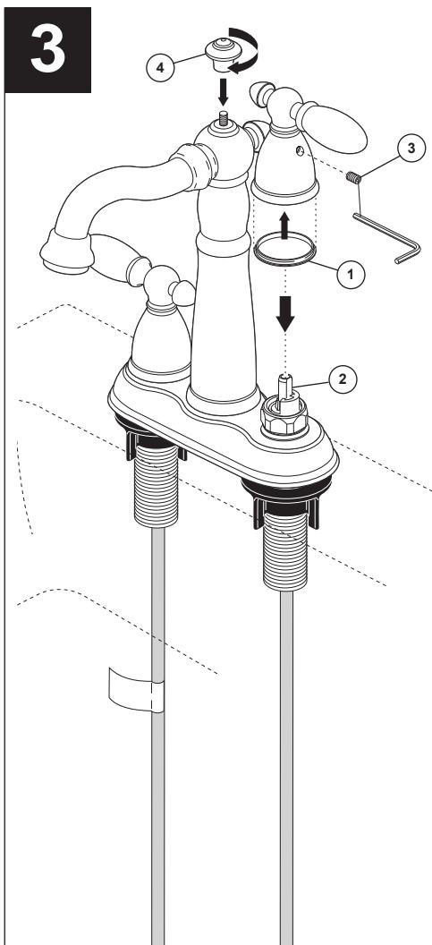
**A.** Remove tube end from slot (1) and fully unwind tube. Repeat for other side.
