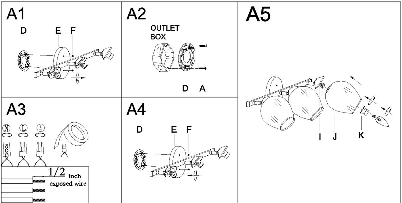
Step A1: Unscrew knob nuts (F) from mounting plate (D), then set them aside for the following steps.
