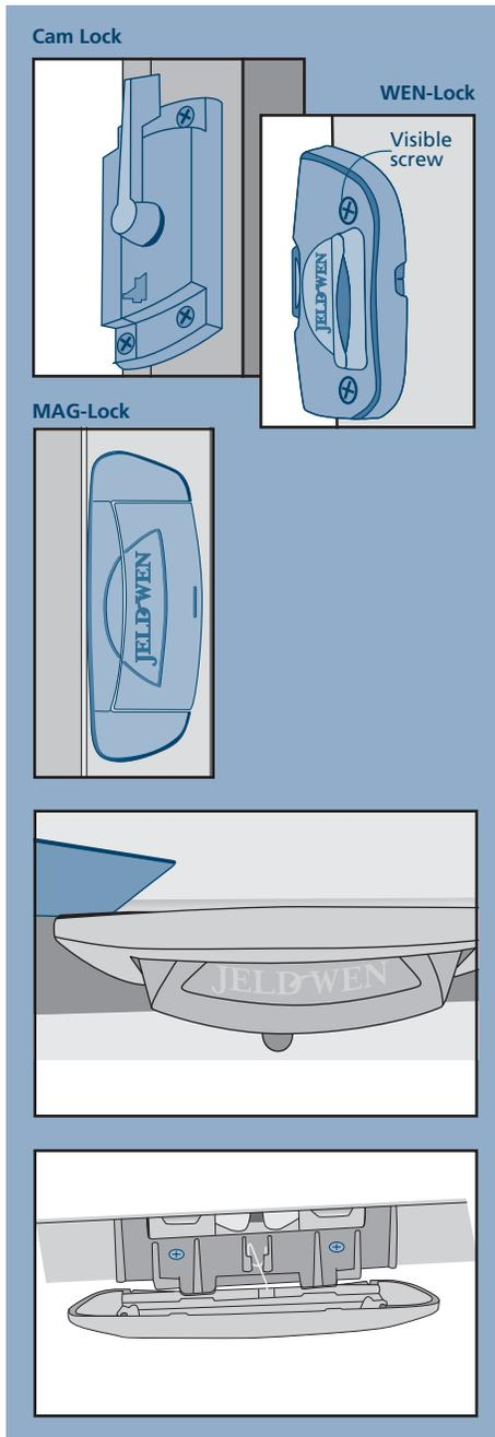
6. Pull up on the handle and slide a putty knife into the gap between the sash and lock on one side. The putty knife will depress a projecting tab on the lock and allow it to be slid out.
