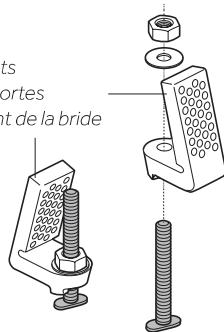
2. Install the bracket onto the flange by inserting the bolt into the large part of the slot. Slide the bracket into the smaller end of the slot and tighten the bolt.
