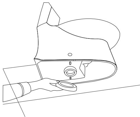
4. Carefully lower the toilet into position so that the brackets are parallel to the inner wall of the toilet. Using a gentle rocking motion, press the bowl down to position the toilet onto the flange and create a seal with the wax ring.
