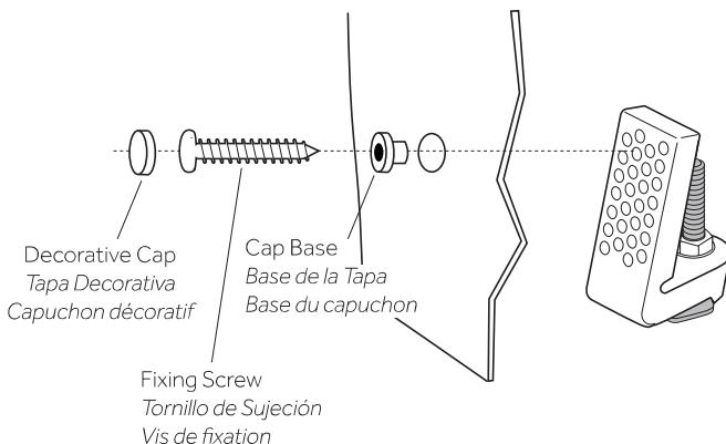
6. Attach the decorative screw cap covers into the mounting holes on both sides of the toilet.
