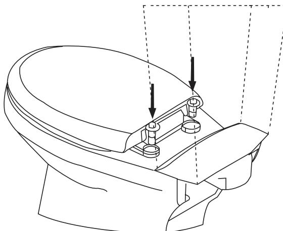
10. Align the toilet seat to the top rim of the toilet bowl. Use a screwdriver to firmly tighten both seat bolts down to the bowl.
