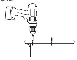
**Step 3** – Pre-drill the handrail for each of the balusters as deep as the length of the baluster screw which is exposed above the wood surface (approx. 3/4") PLUS 1/2"–3/4" to allow for insertion into the rail (1-1/4" — 1-1/2" total). If the baluster screws were installed into the tread, go to step **(4a)**. If the baluster screws were installed into the balusters, go to step **(4b)**.
