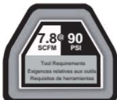
**IMPORTANT:** To operate correctly, this tool requires airflow of at least 7.8 Standard Cubic Feet per Minute (SCFM) at 90 Pounds per Square Inch (PSI) at the tool. The air hose length could affect how much air pressure the tool is actually receiving. You may need to adjust the air pressure higher on the air regulator to achieve the working pressure of 90 PSI.
