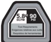
**IMPORTANT:** To operate correctly, this tool requires airflow of at least 5.8 Standard Cubic Feet per Minute (SCFM) at 90 Pounds per Square Inch (PSI) at the tool. The air hose length could affect how much air pressure the tool is actually receiving. You may need to adjust the air pressure higher on the air regulator to achieve the working pressure of 90 PSI.
