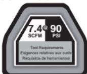
**IMPORTANT:** To operate correctly, this tool requires airflow of at least 7.4 Standard Cubic Feet per Minute (SCFM) at 90 Pounds per Square Inch (PSI) at the tool. The air hose length could affect how much air pressure the tool is actually receiving. You may need to adjust the air pressure higher on the air regulator to achieve the working pressure of 90 PSI.
