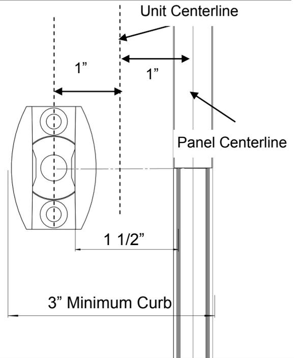
**2\*** Cut the threshold U-channel to the appropriate size. This piece of U-channel will be equal to the opening width. Next drill three 3/16" diameter holes in the center of U-channel (centerline groove provided for convenience), two holes approximately 4-1/2" from each end and one in the middle. Place the U-channel in its correct position with the u-channel centerline over the threshold centerline as marked in step one.
