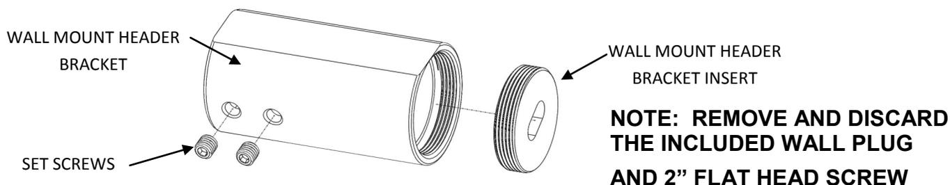
Next, screw the Header Bracket Insert onto the wall with the supplied #10 x 3" Flat Head screw. Install the Header Bracket Insert with the adjustment slot in the vertical direction. This will allow for a small amount of adjustment to make sure the header is level.
