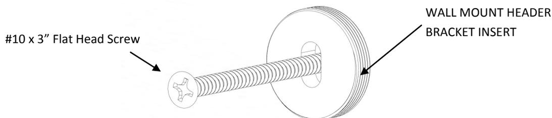
**10** Reassemble the header assembly to the fixed panel glass and the wall mount header bracket. Check the header for level. Lightly tap the wall mount bracket to achieve level. Carefully remove the header assembly and completely tighten the Flat Head Screw from Step 9. Final install the header assembly to the panel glass and wall mount bracket. Tighten the set screws in the wall mount bracket.
