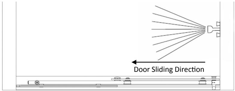
**1** Determine location of the unit centerline on the threshold. From unit centerline mark location of panel centerline 1" towards outside of shower. Next, mark a continuous panel centerline on the wall the panel will mount to, starting where the threshold centerline meets the wall. Use a level to ensure the wall centerline is plumb and straight. The wall centerline should be a minimum of the unit height from the threshold.
