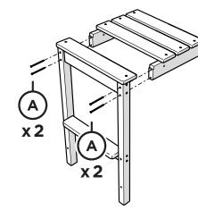
Pre-drilled holes indicate screw placement only. Fully thread screws into material for full engagement
