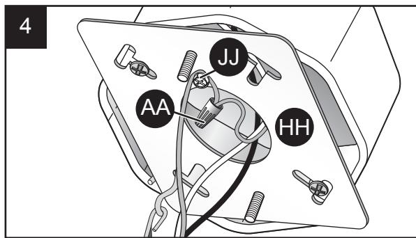
**METAL BOX AND GROUNDED:** If the electrical box is metal and grounded, run the green/copper ground wire attached to the inside of the fixture through the center of the fixture (A) and attach it to the mounting plate (HH) using the grounding screw (JJ).
