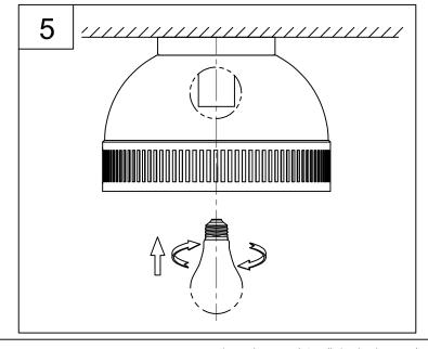
5. Thread the lamp (not included) into the fixture socket. Use 60-watt MAX incandescent medium base lamp, or equivalent SBCFL or SBLED.
