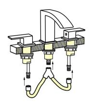
4. Push the blue button on the quick connect hose and insert the hose to the faucet and the handles' pipe as photo 4
