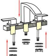
2. Place the faucet body and handles into sink holes, screw the plastic washer, metal washer and locking nut to the thread pipe of the faucet as photo 2
