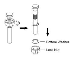
Unscrew the lock nut and bottom washer from drain stopper
