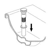
2. Put the pop up drain stopper into sink hole
