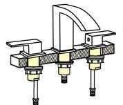
3. Adjust the position of the faucet and the handles then hand tighten the locking nut and then use a screwdriver to tighten the screws on the locking nuts to secure the faucet
