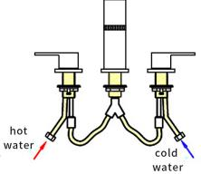
6. Turn on water supply to check for leakage.
