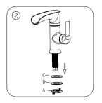
2. Remove the tap and remove the mounting nut (A), metal gasket (B), and rubber gasket (C).
