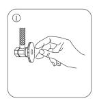
1. Close the water supply valve under the sink or the water in the main water supply area, disconnect the water supply pipe, and remove the old faucet.
