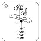
4. From below the sink, slide the rubber gasket (C) and metal gasket (B) onto the tooth tube (4.1) of the body of the faucet, then screw the mounting nut (A) onto the tooth tube (4.1). tighten the mounting nut (A) until the faucet is firmly fixed to the sink.
