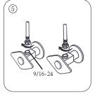
5. Connect the nuts of the hot and cold inlet water hoses to the hot and cold closing valves respectively, and tighten them with a wrench, not too tight. If your water valve is 1 / 2 teeth " please refer to Step 6.
