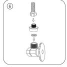
6. Check whether the rubber washer has existed at the end of the rotary joint nut and connect it to the water valve thread connector with a wrench. Connect the nuts of the hot and cold inlet hoses to the rotor on the hot and cold closing valve respectively, and tighten with a wrench, not too tight.
