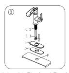
3. Place the bottom plate (D) and panel (E) on the mounting hole of the sink (F), and align the center hole of the bottom plate (D) and panel (E) with the center mounting hole of the sink (F). Pass the water inlet hose (3.1) and the tooth tube (3.2) on the main body of the faucet through the holes in the panel (E), floor (D), and sink (F) until the faucet is placed on the top of the panel (E).
