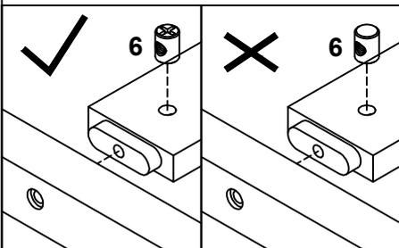
Note: Part 6 will face up with the "x" mark on it, otherwise it cannot be tightened
