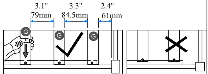
**NOTE:** Please make sure the bed slats close to the side rail before locking the screws to avoid breakage. This step is required for both the left and right sides. Moreover, please do not lock the screws of the bed slats at the outermost edge to avoid damaging.
