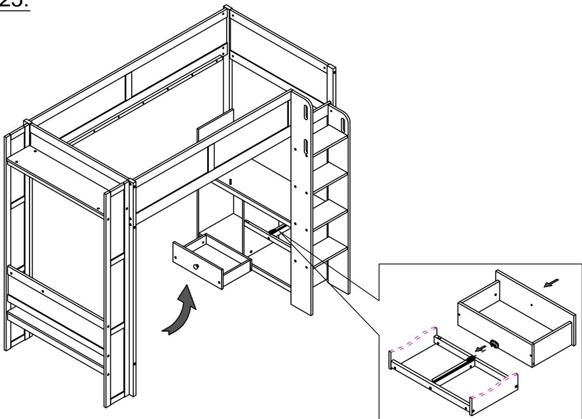
Align the slide rail at the bottom of the drawer and ensure it is secure, then push the drawer in firmly to make the slide rails smoothly on the track.
