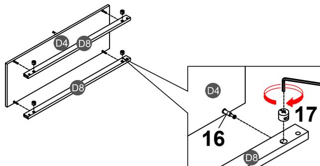
Note: Place hardware #17 with the "X" face outward, and make sure that the arrowhead is upward. Then, place hardware #17 into the hole of hardware #16 and tighten it clockwise with a hand screwdriver. (Please do NOT use an electric screwdriver.)
