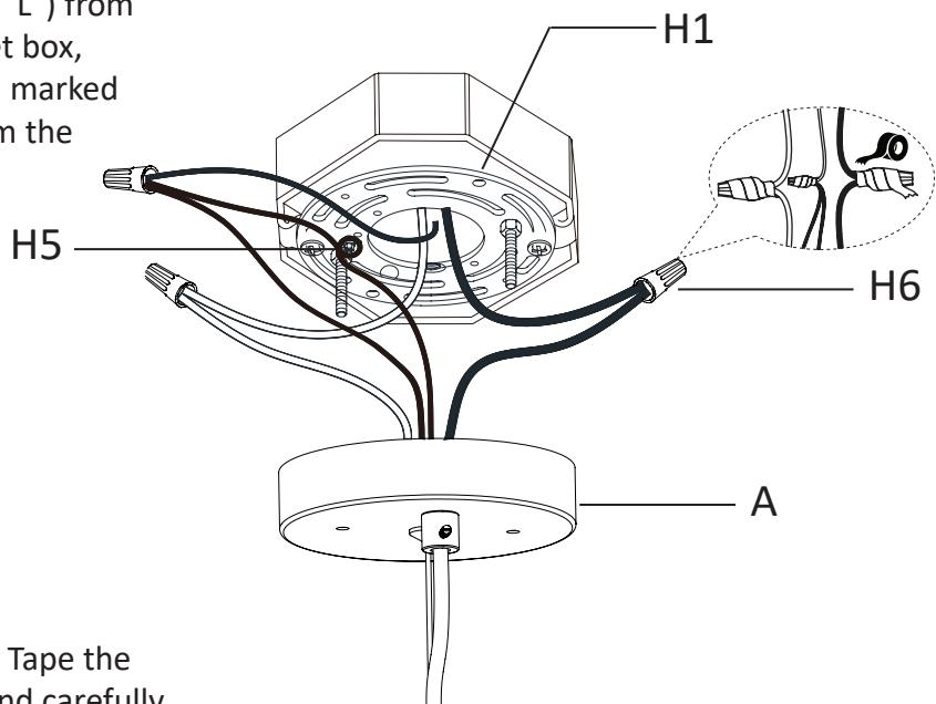
**Note:** Do not let go of the canopy assembly (A) before the canopy assembly (A) installed on the mounting bracket (H1).
