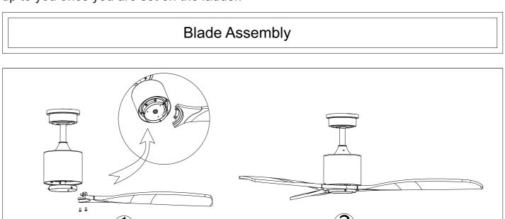
Quick installation: Place a paper pad on each screw and then secure the blade arm to the blade.
