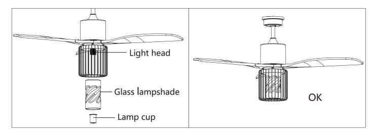
Unscrew the lamp cup from the lamp head first, then put the glass lampshade, and tighten the glass lampshade with the lamp cup.
