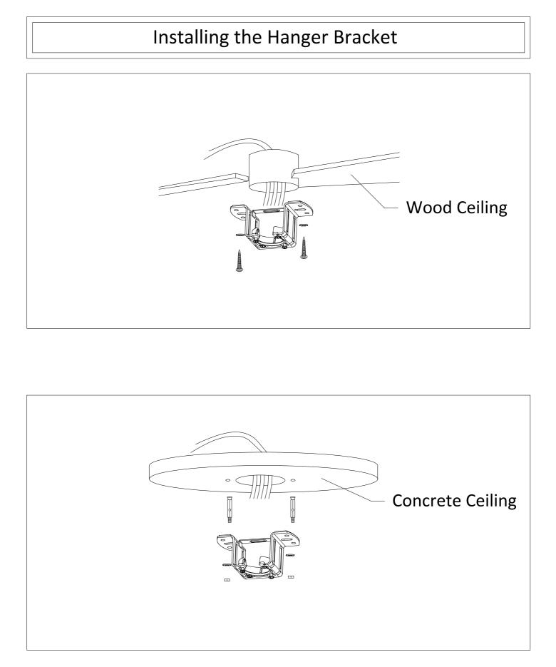
Please drill  $\phi$ 8mm hole on the concrete ceiling, and insert the bolt. Align bracket with the hole, then tighten with nut.
