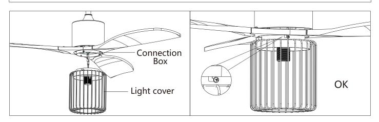
The lampshade is paired with the two lamp lines on the junction box, and pay attention to distinguish the male and the female terminals.
