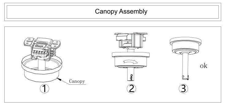
raise canopy to hanging bracket, aligning loosened screws in hanging bracket with slotted holes in canopy. Twist canopy to lock. Re-insert screws and secured all screws with screwdriver.
