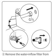
③ Take out the filter by using a flat-blade screwdriver to unscrew the filter
