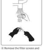
rinse it with clean water (5) Install the filter screen as it is, be sure to tighten it, otherwise it will cause water leakage.
