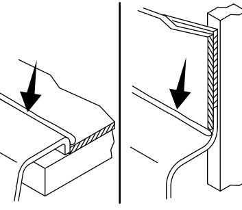
**15** Install the finished deck or wall material to within 1/16" (2 mm) of the bath rim.
