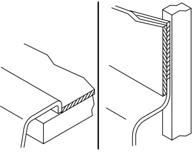
**14** Apply a 1/8" (3 mm) bead of 100% silicone sealant along the seams.
