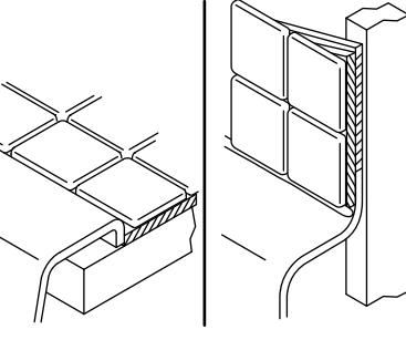
**16** Apply 100% silicone sealant around the bath along the finished deck or walls.
