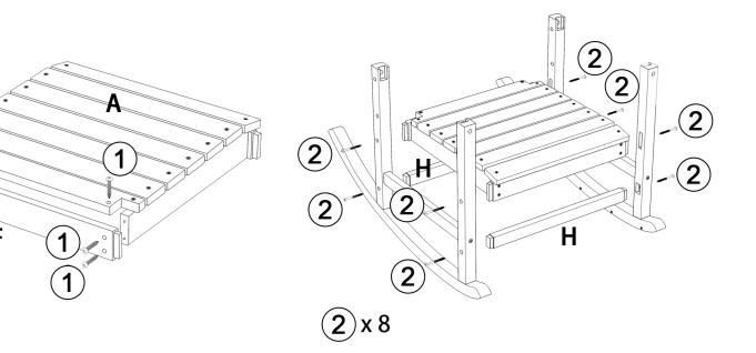
Attach "(F)" to "(A)" - Using "1 M5 × 50MM Screw". tighten with Hex Key. [You've got the "Seat"]
