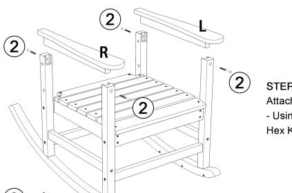
Attach "(L)" and "(R)" to the "Side Frames" - Using "2 M6 × 60MM Screw", tighten with
