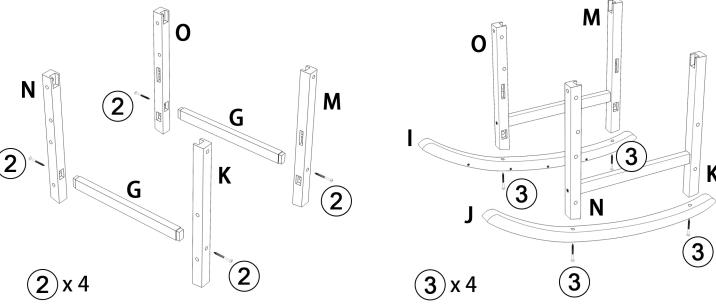
Attach "(G)" to "(N)" and "(K)" - Using "2 M6 × 60MM Screw", tighten with Hex Key.
