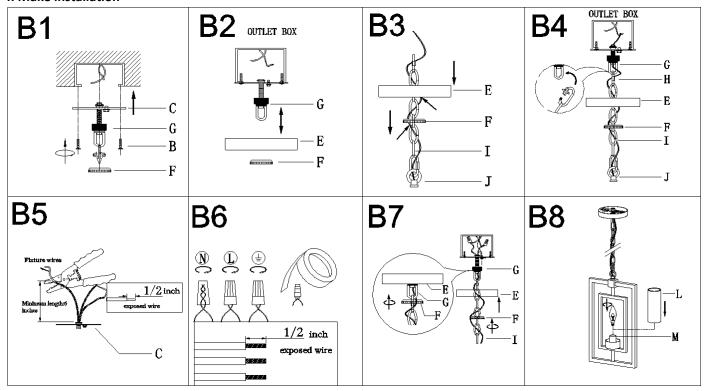
Step B1: Remove collar ring (F) from collar loop (G). Attach single bar (C) to the outlet box with mounting screws (B). Be sure that the side of single bar (C) marked "GND" must face out, then unscrew collar ring (F) from collar loop (G). Step B2: Raise canopy (E) over collar loop (G) and screw collar ring (F) to measure a proper position.
