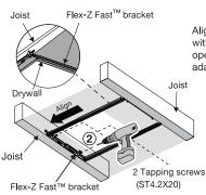
Align the edge of Flex-Z Fast™ with the edge of the ceiling opening on the side where the adapter will be installed.
