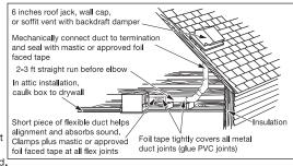
Insulation around the ducts can reduce energy loss and inhibit mold growth. Fans installed with existing ducts may not achieve their rated air flow.
