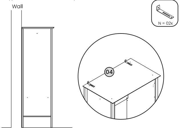
You will need a pencil to mark where you should drill the wall with a 3/8" drill bit to put in the hardware (O).
