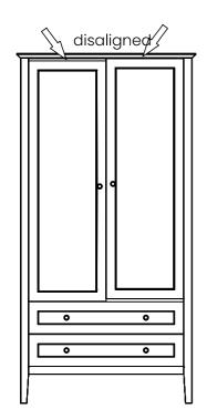
To adjust the alignment of the doors loosen the indicated screw and adjust the 3 hinges up or down on each door, and after aligned, retighten all the screws.
