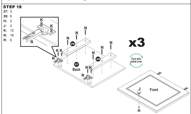
Align two Door Braces (28) with the indents on the backside of Door (27) and secure using six M4.5x25mm Pan Screws (N).
