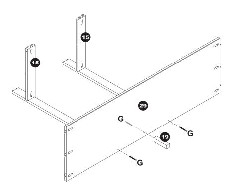
Align the top of Bottom Panel (29) with the back supports, as shown. Secure the bottom panel to each back support using one M4x40mm Flat Screw (G).
