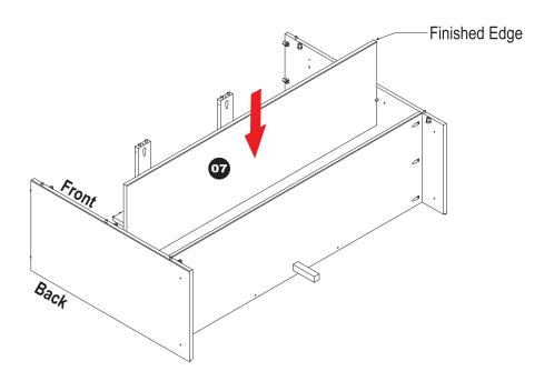
Identify the finished edge of Shelf (07). Slide the shelf into the cabinet, ensuring it is on top of the shelf pins, as shown.
