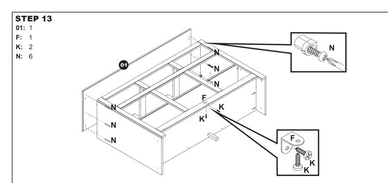
On the bottom of the unit, identify the indent on the backside of the bottom frame and the indent in the bottom, center of the bottom panel. Align one Bracket (F) with the indents and secure using two M3.5x14mm Pan Screws (K).
