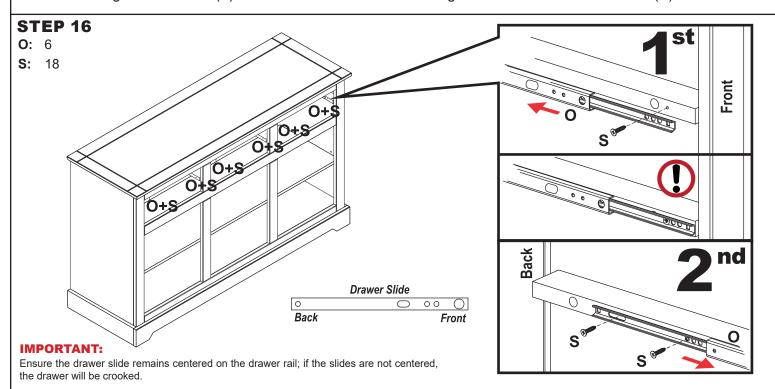
Push the front of Drawer Slide (O) backward. Align the 3rd round hole on the front of the drawer slide with the front indent on the drawer rail and secure using one M3.5x14mm Flat Screw (S).
