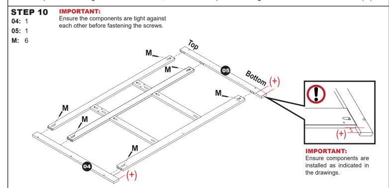
With the dowel mounting holes facing upward, align Right Stile (04), and Left Stile (05), as shown above.
