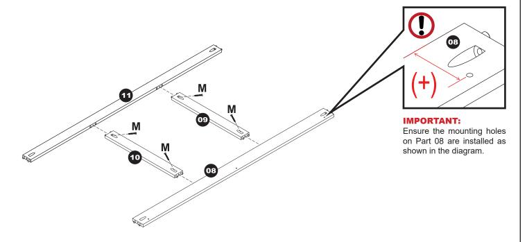
With the angled mounting holes facing upward, align Bottom Frame (08), Left Cabinet Face Frame (09), Right Cabinet Face Frame (10), and Center Face Frame (11) as shown.
