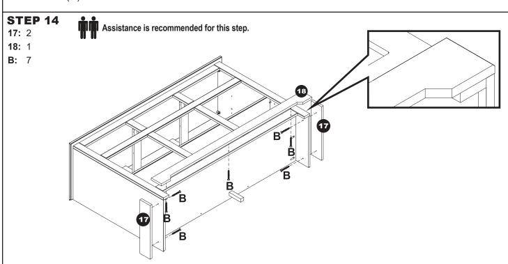
**NOTE:** Have an assistant firmly hold the trim boards in place to ensure they remain flush with the unit while hardware is secured.
