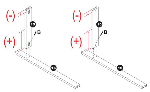
Identify the two indents and the angled pre-drilled holes on Center Drawer Rails (15). Ensuring the indent with the shortest distance from the edge is on top, and the angled pre-drilled holes faces the longer side of the back support, secure Center Drawer Rails (15) onto Back Supports (16) using M4.5x28mm Pan Screws (B).
