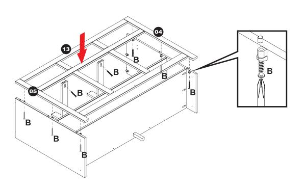
Align the assembled front frame with the cabinet, as shown.
