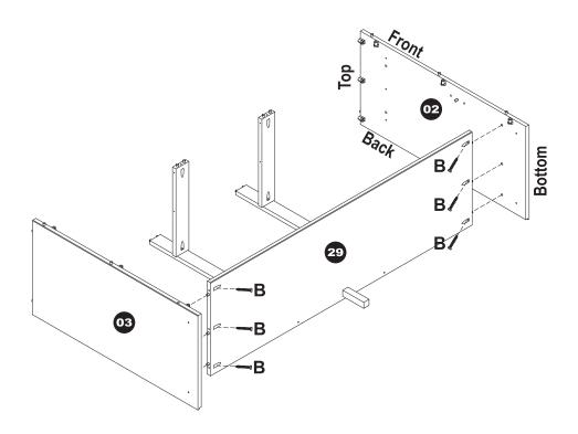
Identify the front, back, top and bottom of Right Side Panel (02) and Left Side Panel (03). Secure each side panel to the bottom panel using three M4.5x28mm Pan Screws (B).
