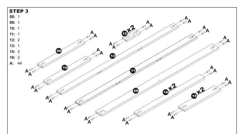
Locate Left Cabinet Bottom Frame (08), Face Frame (09), Right Cabinet Face Frame (10), Center Face Frame (11), two Vertical Drawer Face Frames (12), Top Face Frame (13), two Center Drawer Rails (15), and two Back Supports (16). Install four Wood Dowels (A) into all components, as shown.
