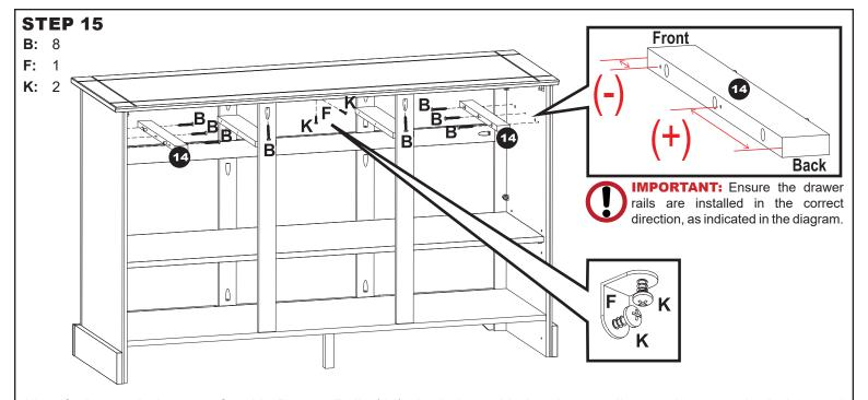
Identify the two indents on Outside Drawer Rails (14), the indent with the shortest distance between the indent and the edge of the rail must be installed toward the <u>front</u> of the cabinet.
