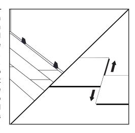
straightness tolerance is within 1/16-in. for lengths over 20-ft. or 1/32 in. for lengths under 20-ft. Complete the following rows starting with a cut piece, such as a piece from a previous row. Install the side joints before the end joints as instructed under "Side Joints" and "End Joints".
