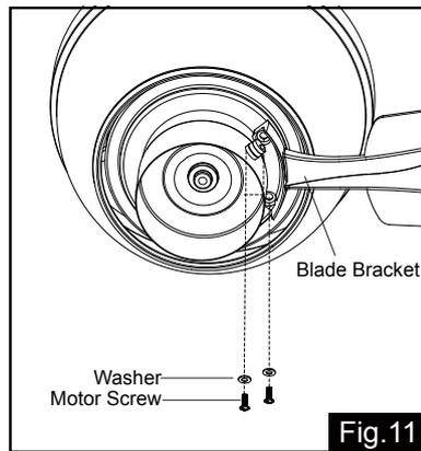
Remove the motor screws and washers from hang motor assembly first. Secure the blade brackets to the motor with motor screws and washers.
