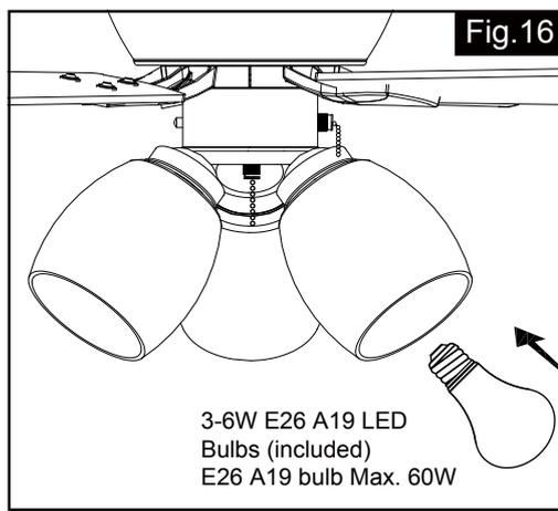
Install LED bulbs (included). See relamping label at socket area or packaging for maximum wattage allowed.
