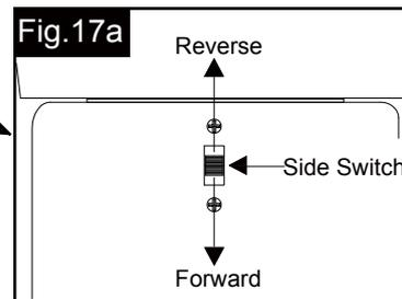
The slide switch on switch box sets direction of fan rotation. Select the desired direction of fan rotation. Push the slide switch down for " Forward" and up for "Reverse".
