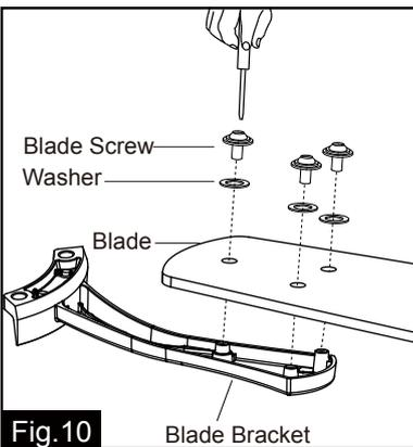
Tighten blades to blade brackets by using blade screws and washers.
