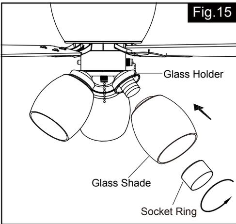
Attach the glass shades onto the glass holders, secure them with socket rings.
