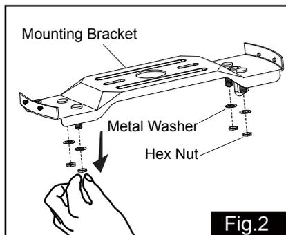
Unscrew the metal washers and hex nuts from mounting bracket. Please save the metal washers and hex nuts for Fig.8 step use.
