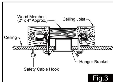
Tighten the hanger bracket to the outlet box with two mounting screws.
