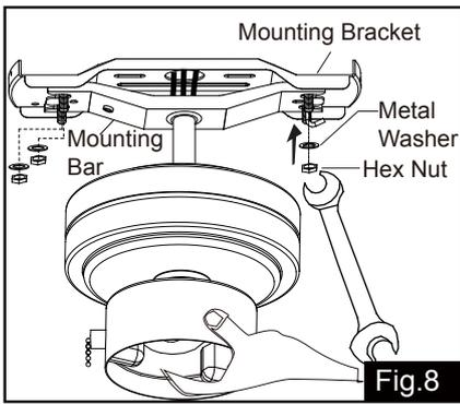
Attach the mounting bar to mounting bracket with metal washers and hex nuts by hand and then free your hands to secure the hex nuts by spanner.
