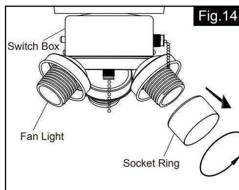
Carefully put the wires into the switch box, then attach the fan light into the switch box with the fan light screws. Remove three socket rings from the fan light for later use.
