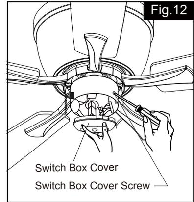
Make sure the wires of the fan light in the switch box are capped with wire connector. Secure the switch box cover into switch box with the switch box cover screws. **To install the fan light, skip this step and proceed to Fig.13.**
