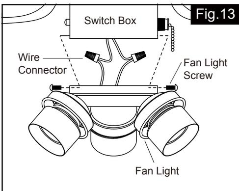
Remove screws from fan light first, then connect the white (neutral) wire from the fan light to white (neutral) wire from switch box with a wire connector, connect the black (hot) wire from fan light to blue (hot) wire from switch box with a wire connector.
