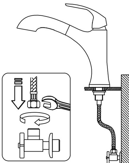
Connect waterlines (5) to angle stops. Tighten both ends of waterlines with a wrench until snug. Turn on hot and cold angle stops and check for leaks.
