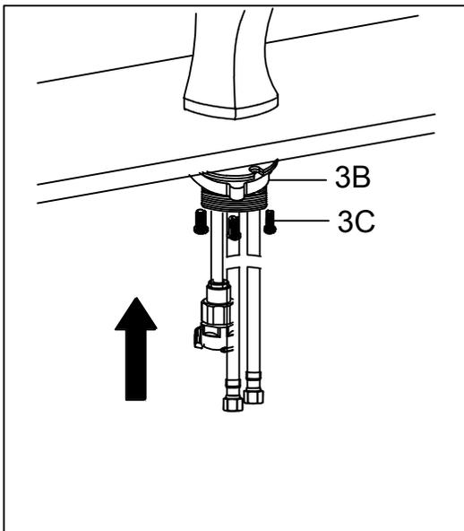
Adjust direction of faucet body (2) so that the faucet is facing straight. Tighten mounting nut (3B) until snug. Tighten mounting screws (3C) to nut with a Phillips screwdriver until snug.
