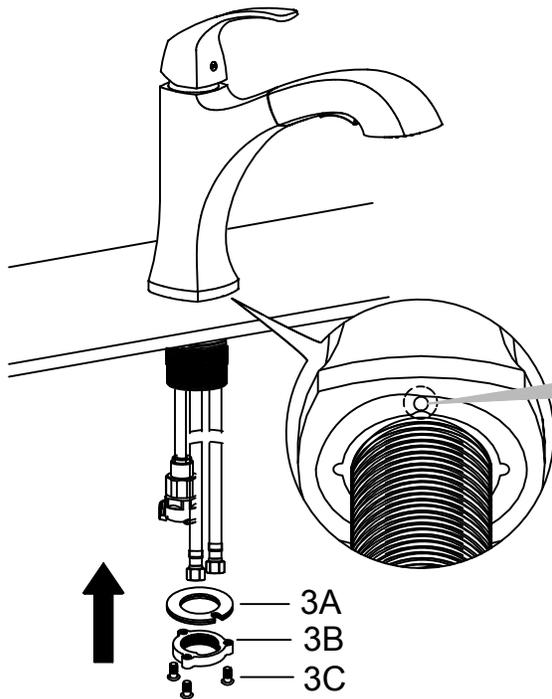
Insert faucet body (2) into hole in countertop or deck plate assembly. Install mounting hardware (3A, B & C) from underneath the countertop.
