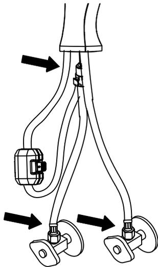
Check for leaks at the connections. Retighten if necessary.
