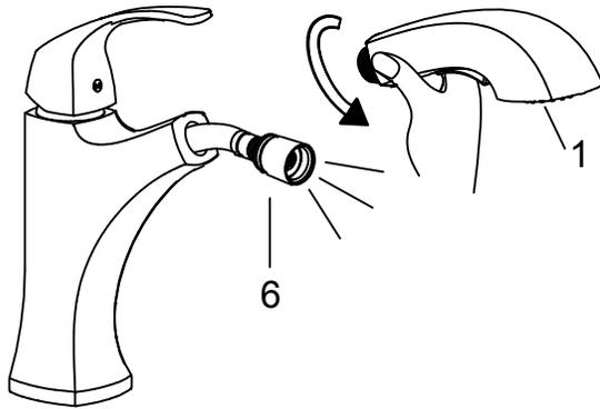
Remove spray head (1) from spray hose (6). Hold tip of spray hose (6). Turn faucet on and let the water run for 60 seconds to flush any debris.
