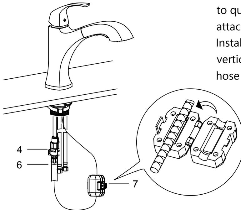
Connect spray hose (6) to quick connector (4) attached to supply line. Install weight (7) on lowest vertical point on spray hose (6).
