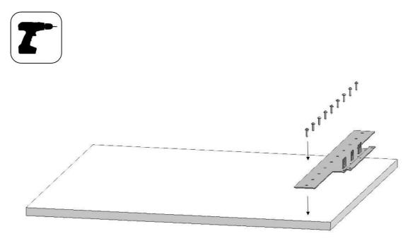
• Attach 3 sheet metal brackets (Item No14) using 6 screws (Item No15) for each.
