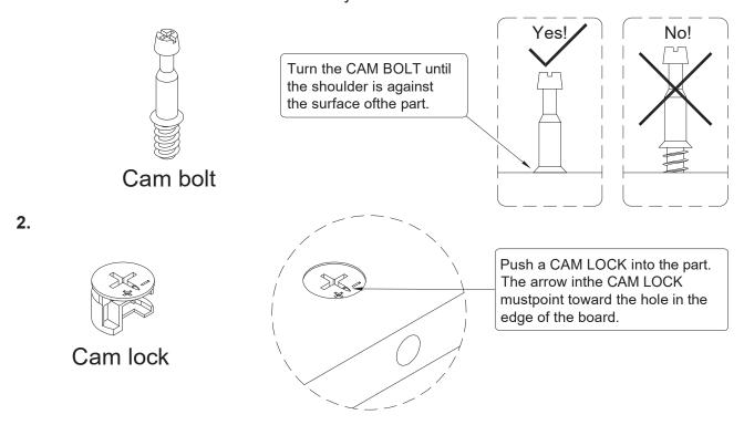
3. Insert the CAM BOLT into the CAM LOCK. Tighten the CAM LOCK.
