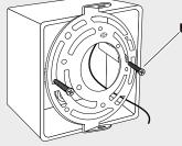
If you install the Mounting Bracket into the electrical box, please use F to fix it instead of E. For your safety, you should use wire connetor A or B as you like, if you choose connector A, you need to use Electric tape for it.
