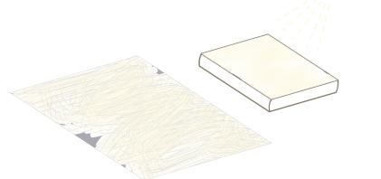
2 Laminate the front surface and cut-out the outside corners as shown
