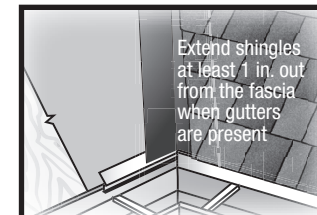
Figure 3L Valley/Shingle Extension
